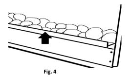
Log & Embers: Once the fire has been installed in the correct position unpack the fuel effect from the accessory box. Place each piece as in the picture below. Do not overlap the front shelf Fig.4. The glass may now be fitted.
